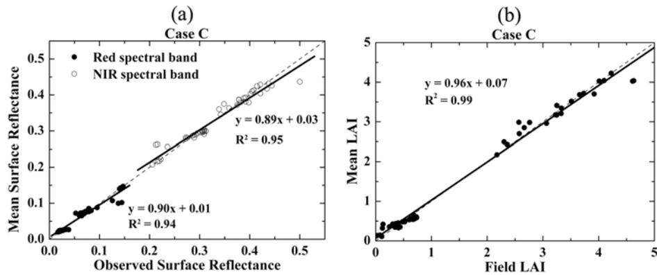
**Figure 7.** (a) Correlation between observed ETM+ surface reflectances and their mean values over corresponding groups. (b) Correlation between field-measured LAIs and their mean values over corresponding groups.
