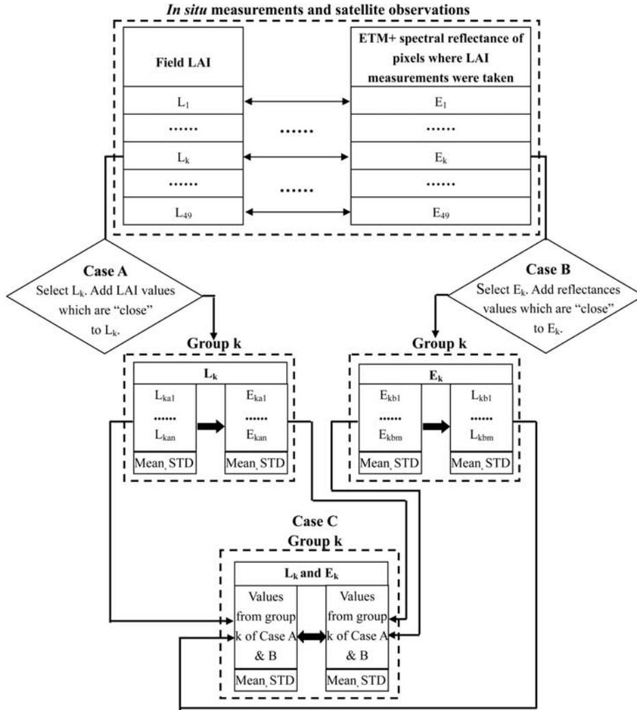
**Figure 3.** Derivation of reference values. Group  $k$  in case A consists of pairs of measured LAI values  $L_{kai}$  which are “close” to  $L_k$  and corresponding ETM+ surface reflectances  $E_{kai}$ . Similarly, group  $k$  in case B includes ETM+ surface reflectances  $E_{kbi}$  being “close” to  $E_k$  and respective measured LAI values  $L_{kbi}$ . Group  $k$  in case C is obtained by merging groups  $k$  in cases A and B.
