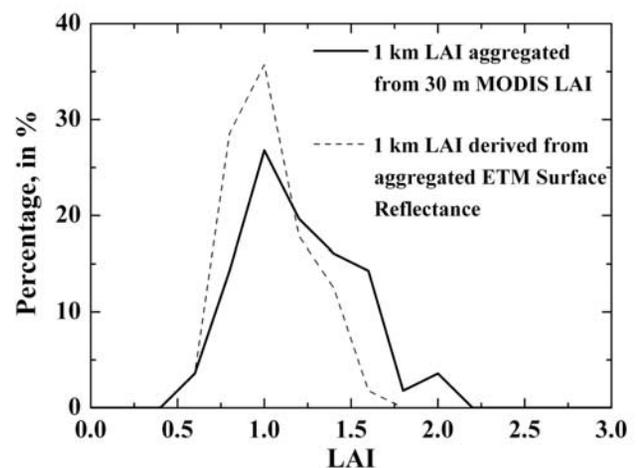
**Figure 11.** Plot of LAI values at 1 km resolution obtained by (1) averaging 30 m resolution LAI retrievals (solid line) and (2) applying the MODIS operational algorithm to 1 km surface reflectance aggregated from 30 m ETM+ data (dashed line).
