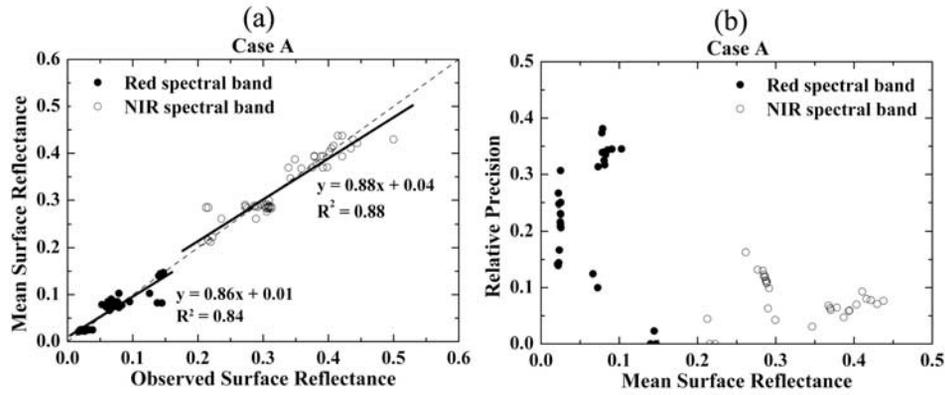
**Figure 4.** (a) Correlation between observed surface reflectances and mean values over associated groups for red (solid circles) and NIR (open circles) wavelength. (b) Relative precision of the mean surface reflectance in the red (solid circles) and NIR (open circles) spectral bands.
