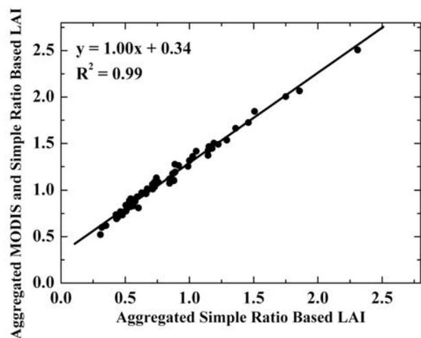
**Figure 13.** Correlation between 1 km LAI maps obtained by averaging 30 m simple ratio–based retrievals and 30 m MODIS LAI amplified with the adjusted simple ratio–based LAI.
