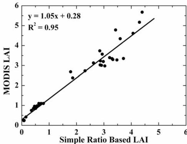
**Figure 10.** Correlation between LAI values derived from the simple ratio-based technique and the MODIS LAI and FPAR algorithms.
