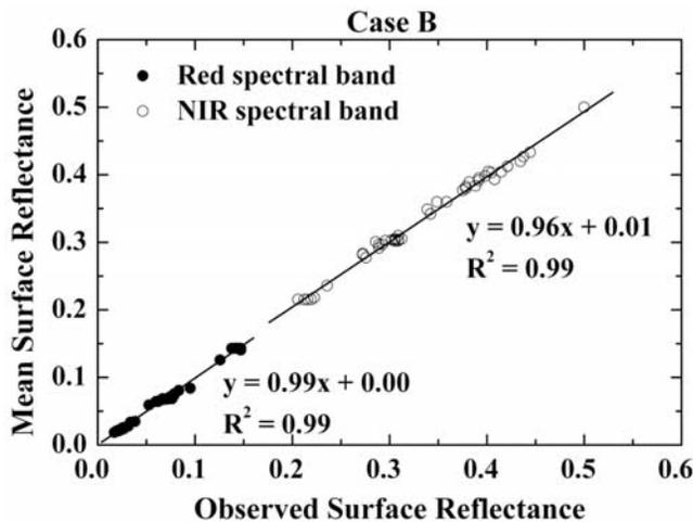
**Figure 5.** Correlation between observed ETM+ surface reflectance and its mean over “indistinguishable” observations for red and NIR spectral bands.
