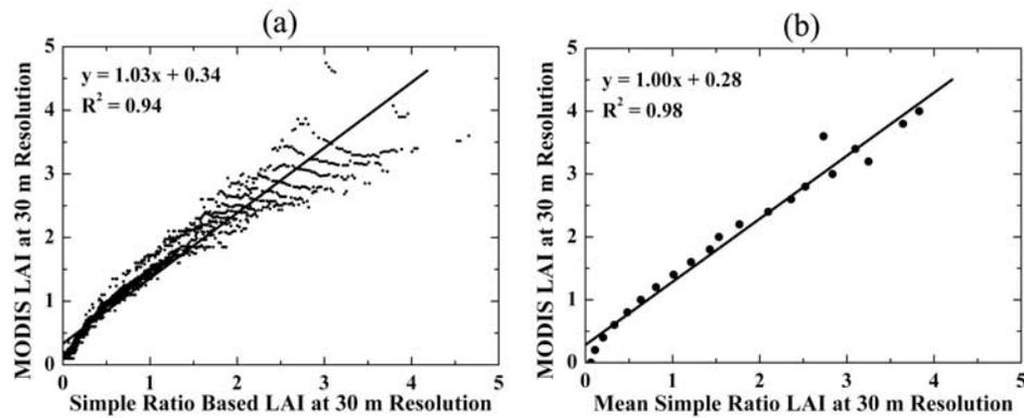
**Figure 12.** (a) Correlation between LAI values produced by the simple ratio–based technique (SR LAI) and the 30 m resolution MODIS LAI and FPAR algorithm for a  $10 \times 10$  km area centered on the remote sensing data assimilation experiment site. (b) Correlation between the mean SR LAI and MODIS retrievals. The mean values are obtained by averaging SR LAIs corresponding to a given value of the MODIS LAI.
