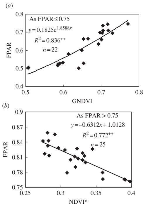
Figure 4. Hyperspectral VI-based estimation models of fraction of photosynthetically active radiation (FPAR) absorbed by corn canopies. Shown here are (a) GNDVI–FPAR model ( $FPAR \leq 0.75$ ) and (b) NDVI\*–FPAR model ( $FPAR > 0.75$ ).
